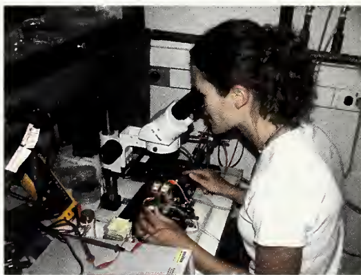
Figure 1. Elizabeth Mirowski characterizing spin-valve magnetic traps for microfluidic magnetic bead capture and sorting.
